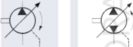
Variable Displacement Pump, external case drain (from left to right: single flow direction, two flow direction)
