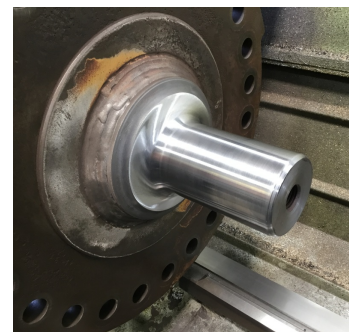
Condition of end cap and trunnion mount post final machining
